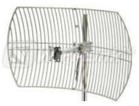
Square grid antenna is designed for the spread spectrum system, the surface design with welded-steel reflector to bring out the best performance. This antenna features high gain, long coverage, light weight, compact structure and excellent wind-resistance. It is used for outdoor and the range is up to 6.2 miles.
