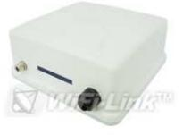
This panel antenna delivers extended access point range in a single floor environment ideally positioned in the corner of a building. It functions from point-to-point so that you can wirelessly connect LANs between the buildings in a campus-type environment. It provides multiform transmission when placed on a Wall, as the higher powder output extends the range through typical flooring materials
